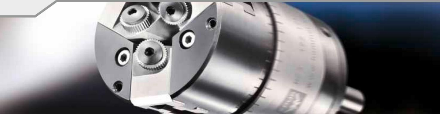
The zeus® RF3 series is designed for the fine machining of very small and thin-walled work pieces in axial tool direction. The product series is suitable for producing straight and RGE profiles with high demands on surface quality and dimensional accuracy. Due to the special design with three knurling wheels operating, the lateral pressure is reduced to a minimum. zeus® RF3: A specialist for knurling thin or pressure-sensitive parts, as for example spindles, tubes, or delicate bushings.
